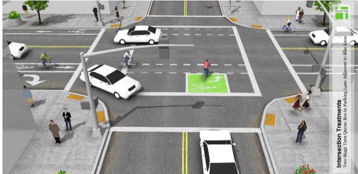
Figure 22 Two-Stage Turn Box Design
