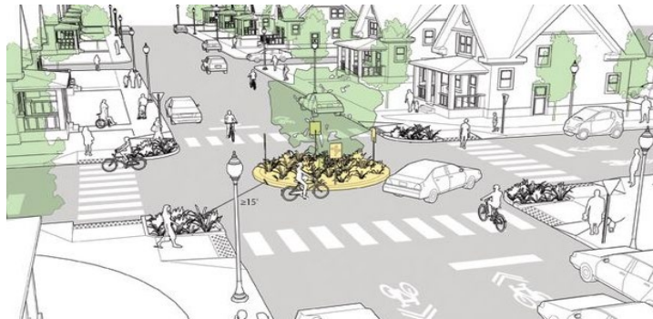
Figure 24 Diagram of a Traffic Circle
