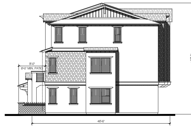
BUILDING A RIGHT ELEVATION
