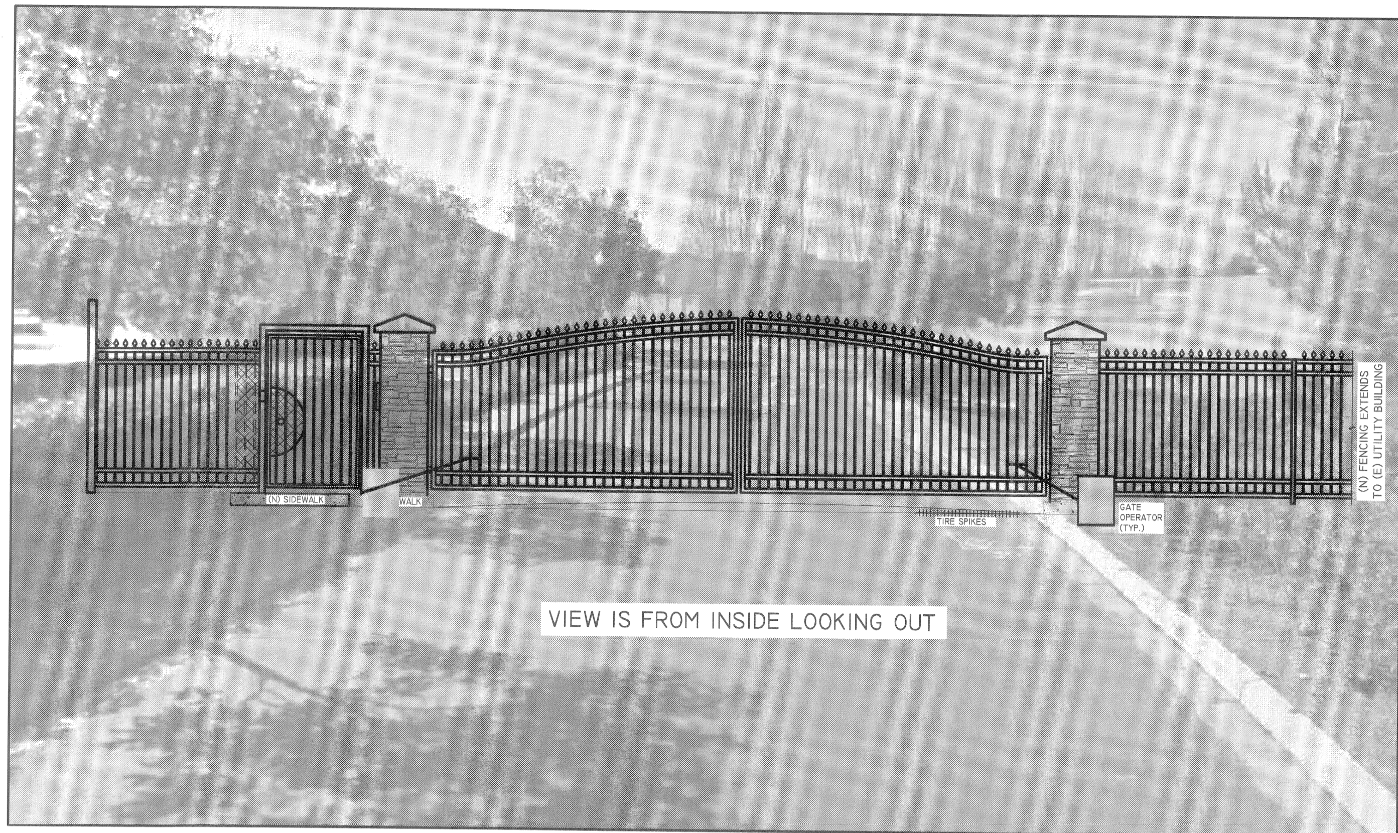
1 VISITOR'S ENTRANCE GATE, PARTIAL FENCING, & SIGNAGE - SITE ELEVATION 1/4" = 1'-0"
