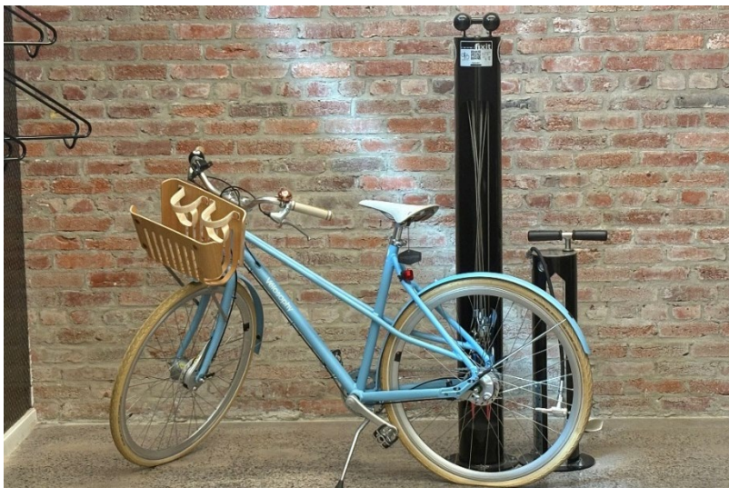
A basic bicycle repair station includes an air pump, a bicycle stand, and a set of standard bicycle tools for maintenance and repair.
