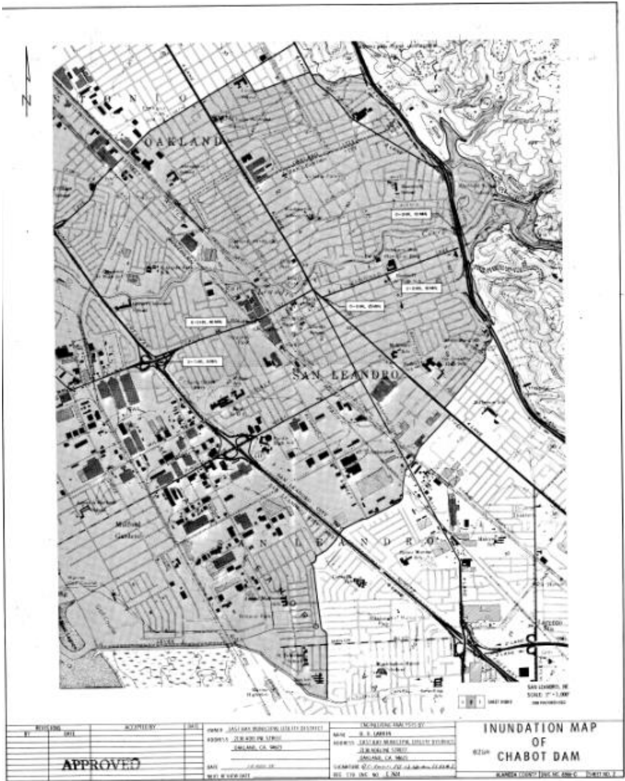
Figure 5-15 Dam Failure Inundation Map 1 of 2 – CAL OES
