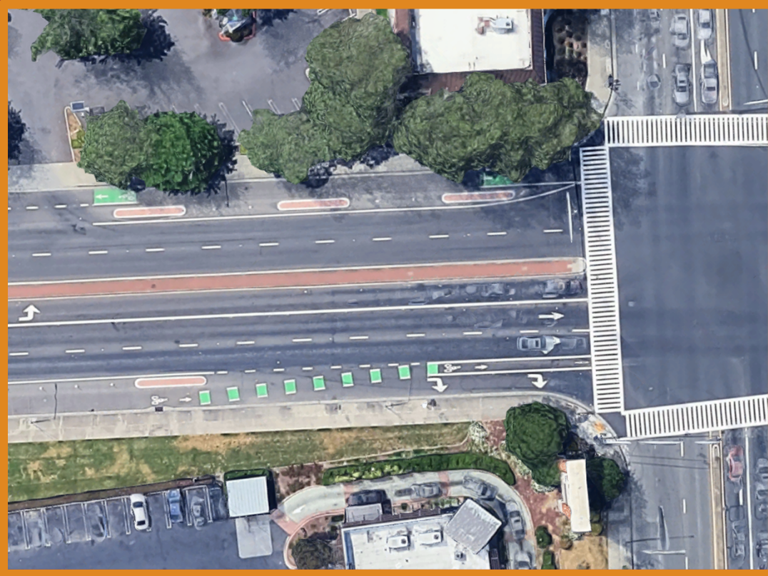
Dashed Green Conflict Zone Striping
