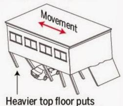
Heavier top floor puts disproportionate lateral stress to the soft story causing a possible collapse.
