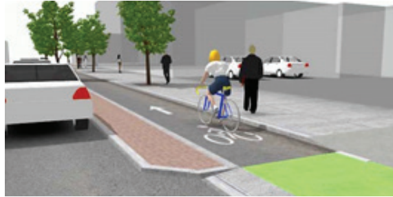
Example of raised Class IV one-way cycle track (NACTO Urban Bikeway Design Guide)
