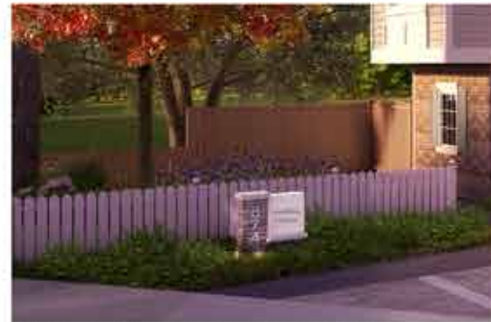
3'-0" FENCE - PRESSURE TREATED WOOD - WHITE PAINT 6'-0" FENCE - PRESSURE TREATED WOOD - TRANSPARENT STAIN FINISH
