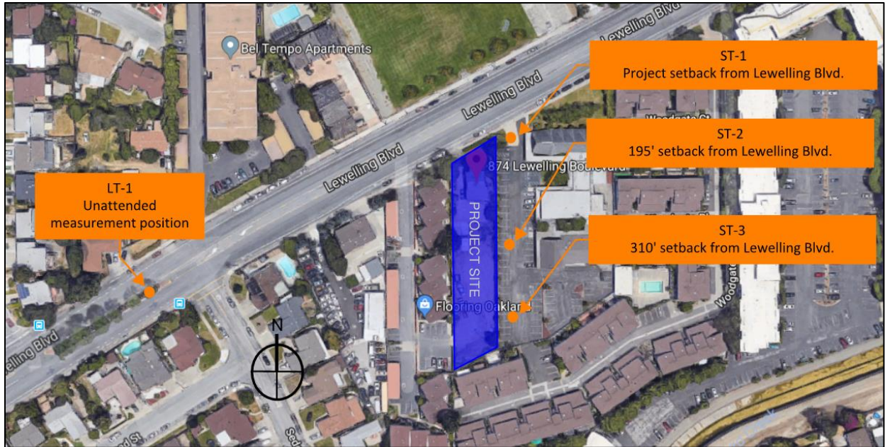
Figure 1 – Noise Survey Measurement Positions
