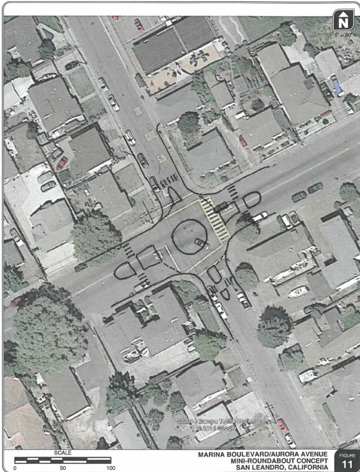
Figure 11 Preliminary Drawing of a Modern Mini-Roundabout
