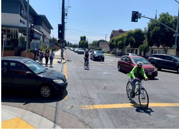
Left to right: (1) People bike through the busy intersection of Estudillo Avenue, which has an 85th percentile speed of 34 mph and lacks bicycle crossing or turning facilities. (2) Standard bike lanes run along Doolittle Drive, which is a street that intersects with rail tracks and frequently sees truck traffic.
