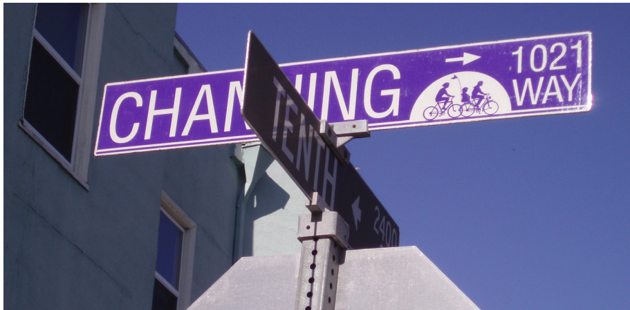
In Berkeley, bicycle boulevards have modified street signs (standard on bottom, bicycle boulevard on top) that indicates its status as a bicycle boulevard to all road users.
