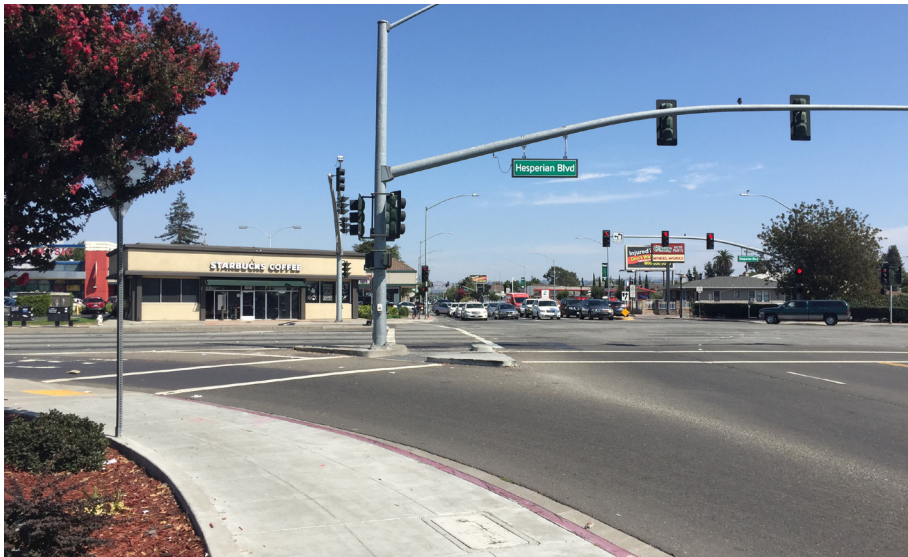
A free right turn lane at the intersection of Hesperian Boulevard and Lewelling Boulevard.
