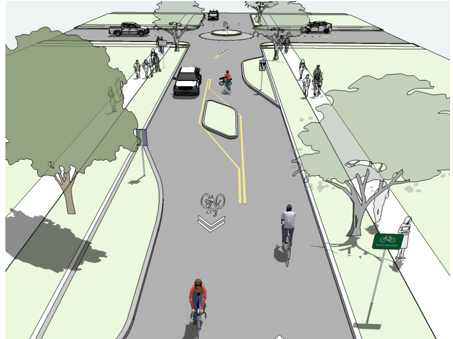
This Class III illustration shows many potential road diet techniques including sharrows, median islands, chicanes, and mini-roundabouts; this illustration is not inclusive of all treatments. Specific treatments should be determined on a street-by-street basis.
