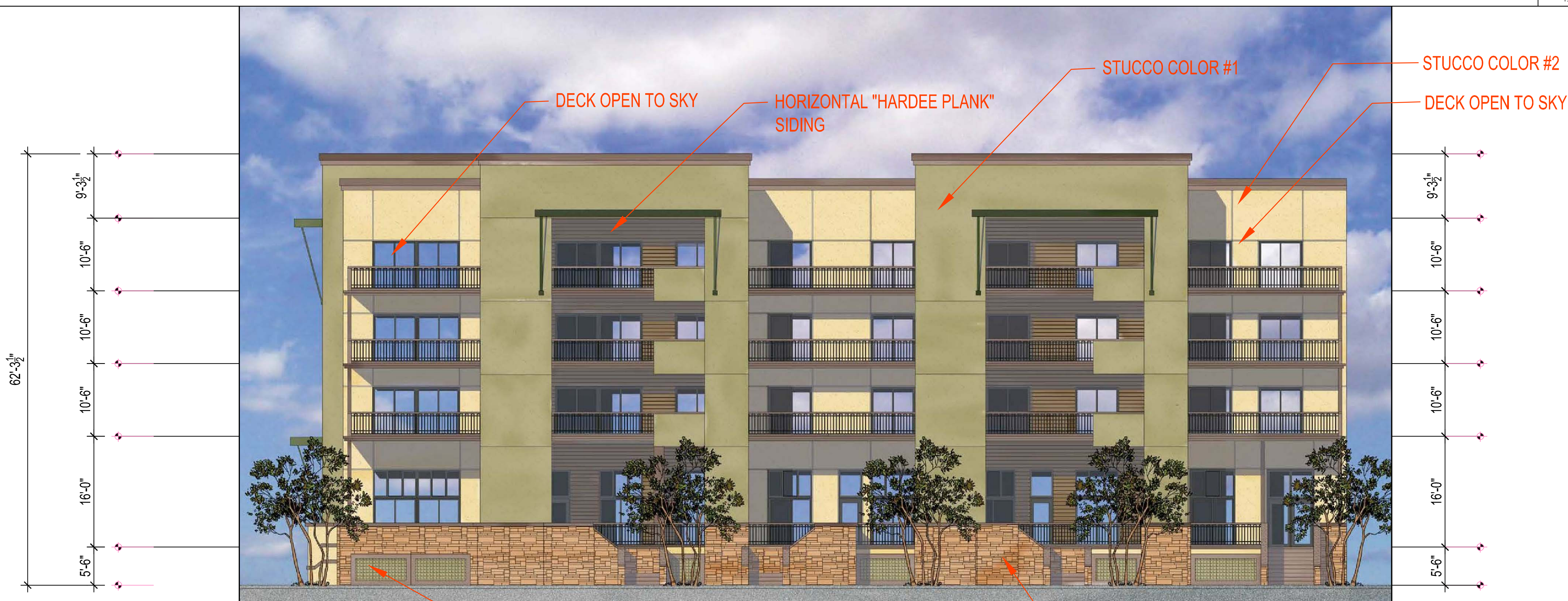
EAST ELEVATION FACING WASHINGTON AVENUE
