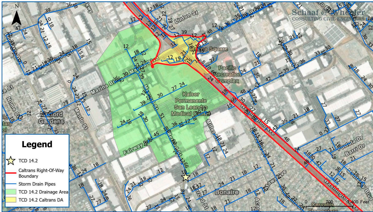
Figure 4: Site 14.2 Drainage Area
