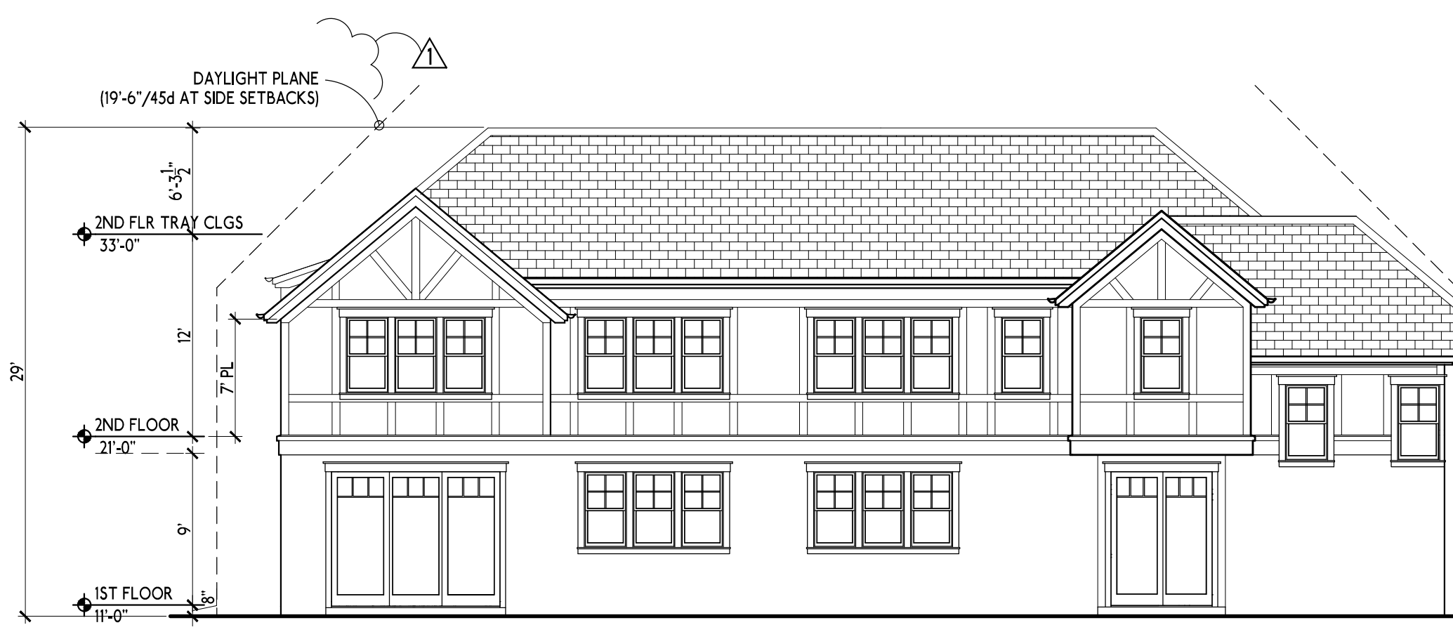
NEW DUPLEX REAR (SOUTH) ELEVATION
