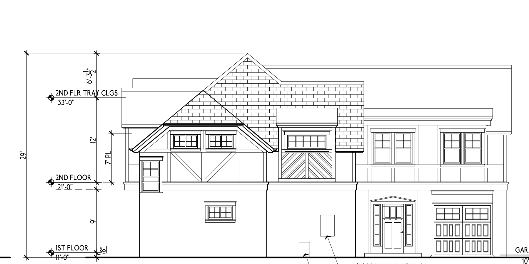
NEW DUPLEX LEFT (EAST) ELEVATION
