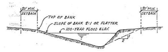
**Section B** — Typical where existing channel is sufficiently large to allow side encroachment.
