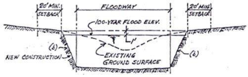
**(b)** = Sides of channel shall be structurally stable. If sides are of earth, they shall have a maximum slope of 2 horizontal to 1 vertical.
