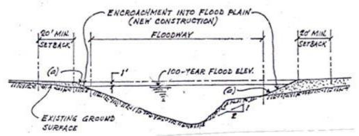
(a) = Slope of bank shall be 2 horizontal to 1 vertical or flatter, as determined by director of public works.
