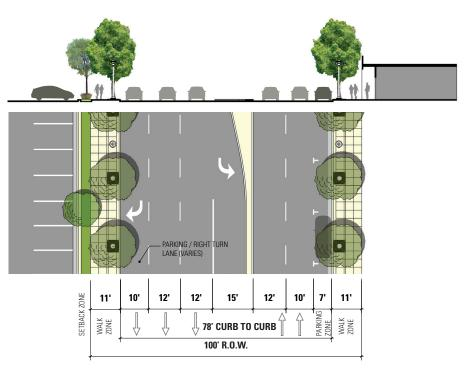
Figure 3.4: Existing East 14th Street Cross Section
