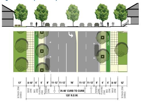
\*Note: the design of the proposed Hesperian street section may be adjusted along different street segments and at approaches to intersections
