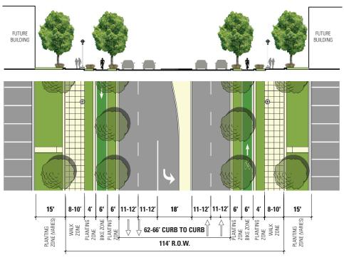
\*Note: The design of the proposed Fairmont street section may be adjusted along different street segments and at approaches to intersections
